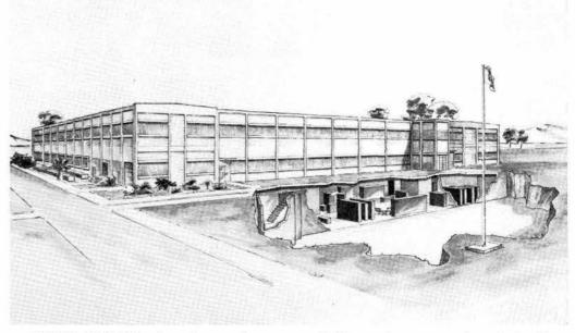
ARTIST'S CONCEPT of underground computer facility under construction at Sandia Laboratories Livermore shows relocation of equipment after site is completed in November 1969. The new facility will house three computers—a CDC 6600 and 3600, and an IBM 1401.
